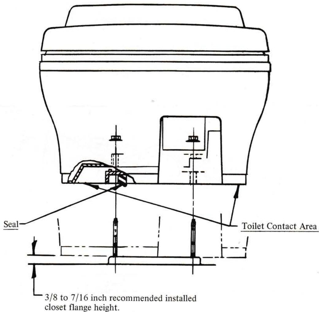
Lay a straight edge across closet flange and measure distance to floor at toilet contact area to check flange installation. Too much gap may cause the flush mechanism to bind. Too little gap may prevent a good seal.
